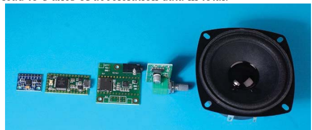
Figure 1: The electronic parts of the “Motion Sound Box” (Copyright: Thomas Bisitz)
