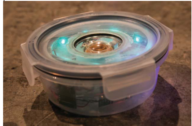
Figure 3: Prototip with LED illumination in transparent case and loudspeaker with transparent membrane (Copyright Theo Stenert)
